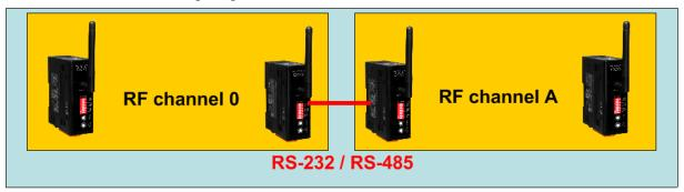
Using two RFU-400s, connect their RS-232 or RS-485 to each other, as shown in the middle of the figure above. So that you can form a group of RFU-400 repeaters to extend the wireless communication distance.
